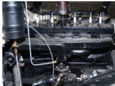
The 218.6-cu.-in. inline six produces 68 horsepower.
